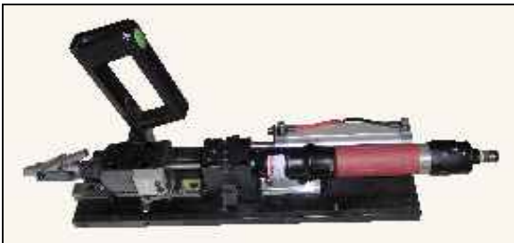
Slide 5100 double stroke with pneumatic screwdriver and handle
