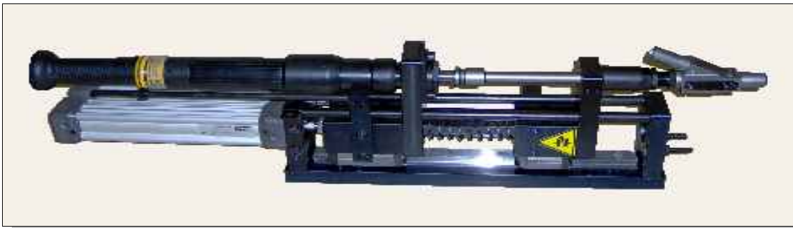
Slide 4900 double stroke 160mm with screw jam eject cylinder and electronic screwdriver
